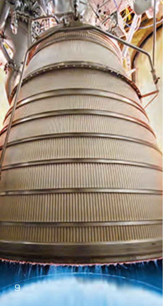
Atlas V Depending on mission requirements, the United Launch Alliance Atlas V's Centaur upper stage is powered by a single RL10C-1 engine or two RL10A-4-2 engines.
