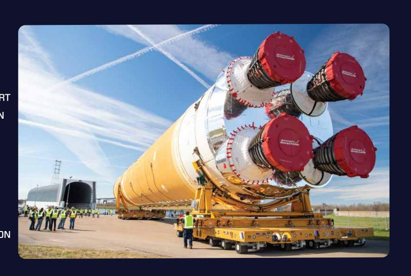
Upgraded for SLS from the Space Shuttle program, engines 2045, 2056, 2058 and 2060 will support the first SLS flight, Artemis I, and the Core Stage Green Run test. These four flight proven engines contributed to 21 successful Space Shuttle flights for more than three decades. Two of the engines supported the last Space Shuttle mission, STS-135, and now they will usher in a new era of exploration.
